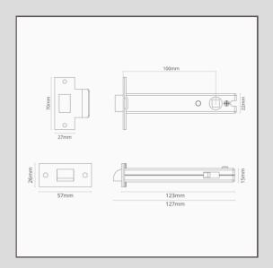
Our light latch will keep your door tightly closed. It's engineered with light springs, so it's ideal for use with sprung lever door handles and unsprung door knobs.
