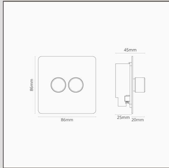
Powered by the latest technology, this rotary style Dimmer Switch lets you set the mood on two different lights.
