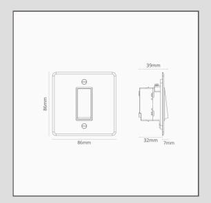
This one-gang centre-retractive rocker switch in polished nickel is a more modern alternative to our toggle switches.
